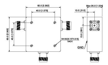
Unit: mm [inch] Tolerance: ±0.2mm
